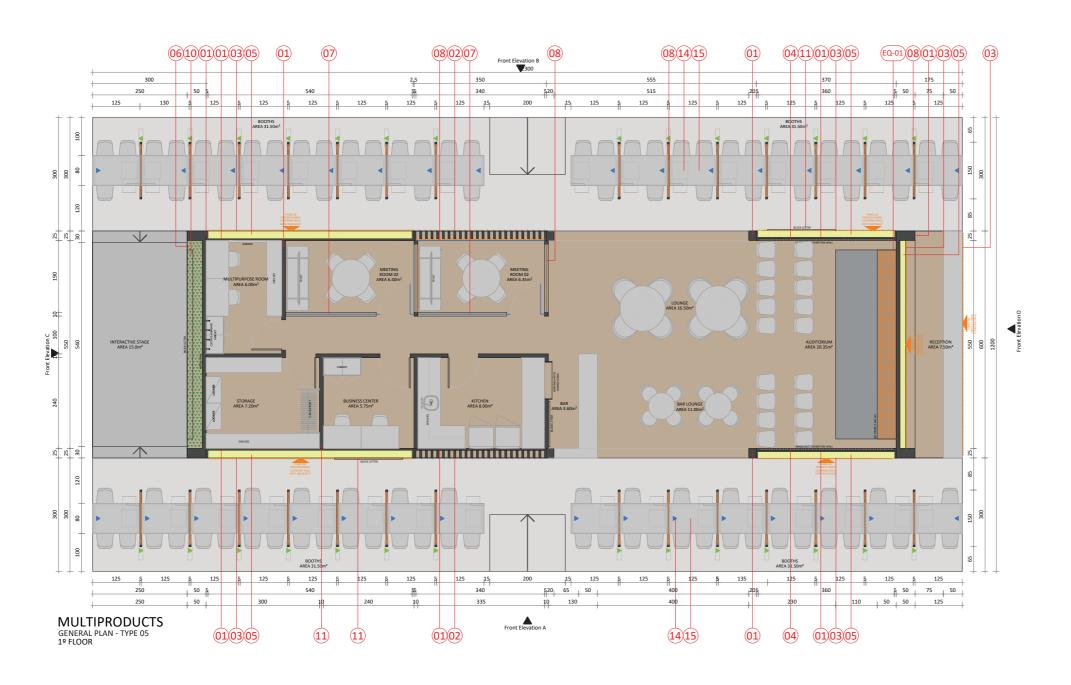
Modular system structure (preferably BeMatrix system, or similar) that uses in its structural system frame with aluminum profiles of at least 52mm wide and its superior multiples. Finishing cover in rigid panel must be fastened with velcro tape over the modular structure. Finishing cover in reforestation pinus plywood panel with varish finishing or MDF sheet with colored melanin finishing.
